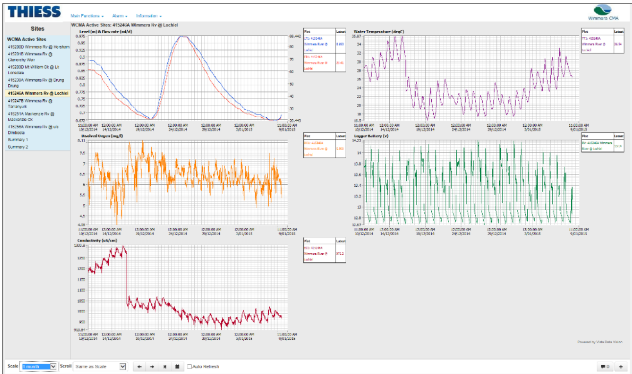
Figure 9-1. Telemetry provides instantaneous measures of flow rates and various water quality parameters at key sites across the Wimmera River System.
