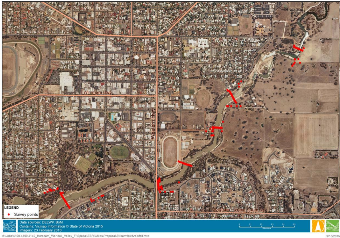
Figure 5-3 Wimmera River cross section survey
