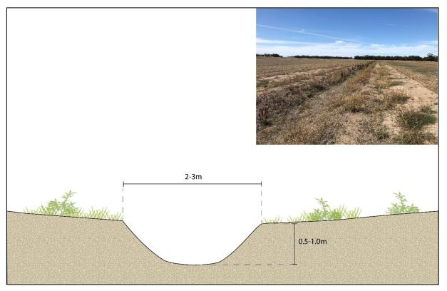
FIGURE 5-29 DUNMUNKLE CREEK CHANNEL DIMENSIONS IN THE LOWER REACH, WHERE AN OBVIOUS SPOIL MOUND IS NOT PRESENT.
