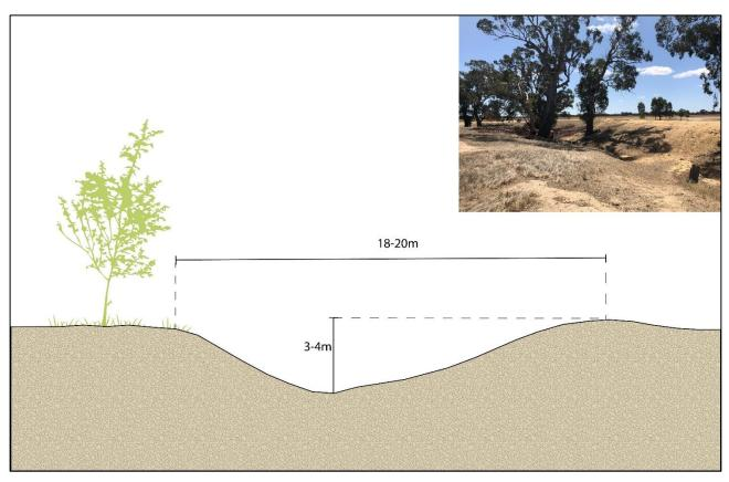
FIGURE 5-5 TYPICAL CHANNEL DIMENSIONS IN THE UPPER REACH EXCLUDING WHERE THE CHANNEL INHERITS PALAEOCHANNELS OF THE WIMMERA RIVER.
