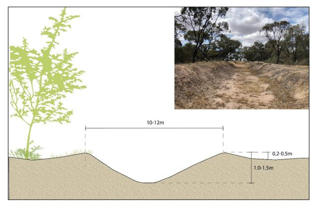
FIGURE 5-28 TYPICAL CHANNEL DIMENSIONS IN THE LOWER REACH OF DUNMUNKLE CREEK, SHOWING THE SPOIL MOUNDS THAT HAVE FORMED LEVEES.
