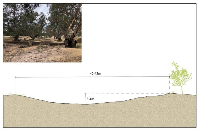
FIGURE 5-4 TYPICAL CHANNEL DIMENSIONS OF DUNMUNKLE CREEK WHERE THE CHANNEL INHERITS PALAEOCHANNELS OF THE WIMMERA RIVER.
