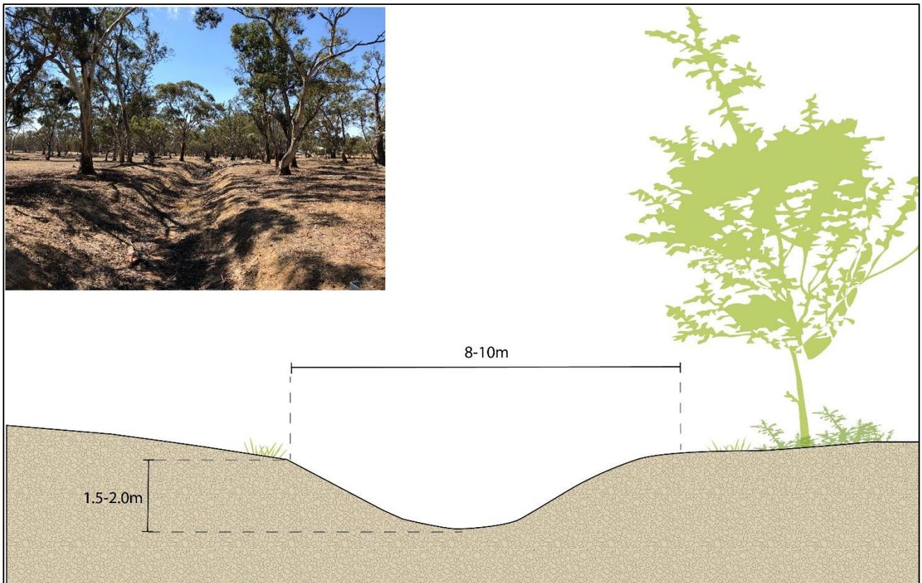
**FIGURE 5-17 TYPICAL CHANNEL DIMENSIONS OF DUNMUNKLE CREEK IN THE MIDDLE REACH.**
