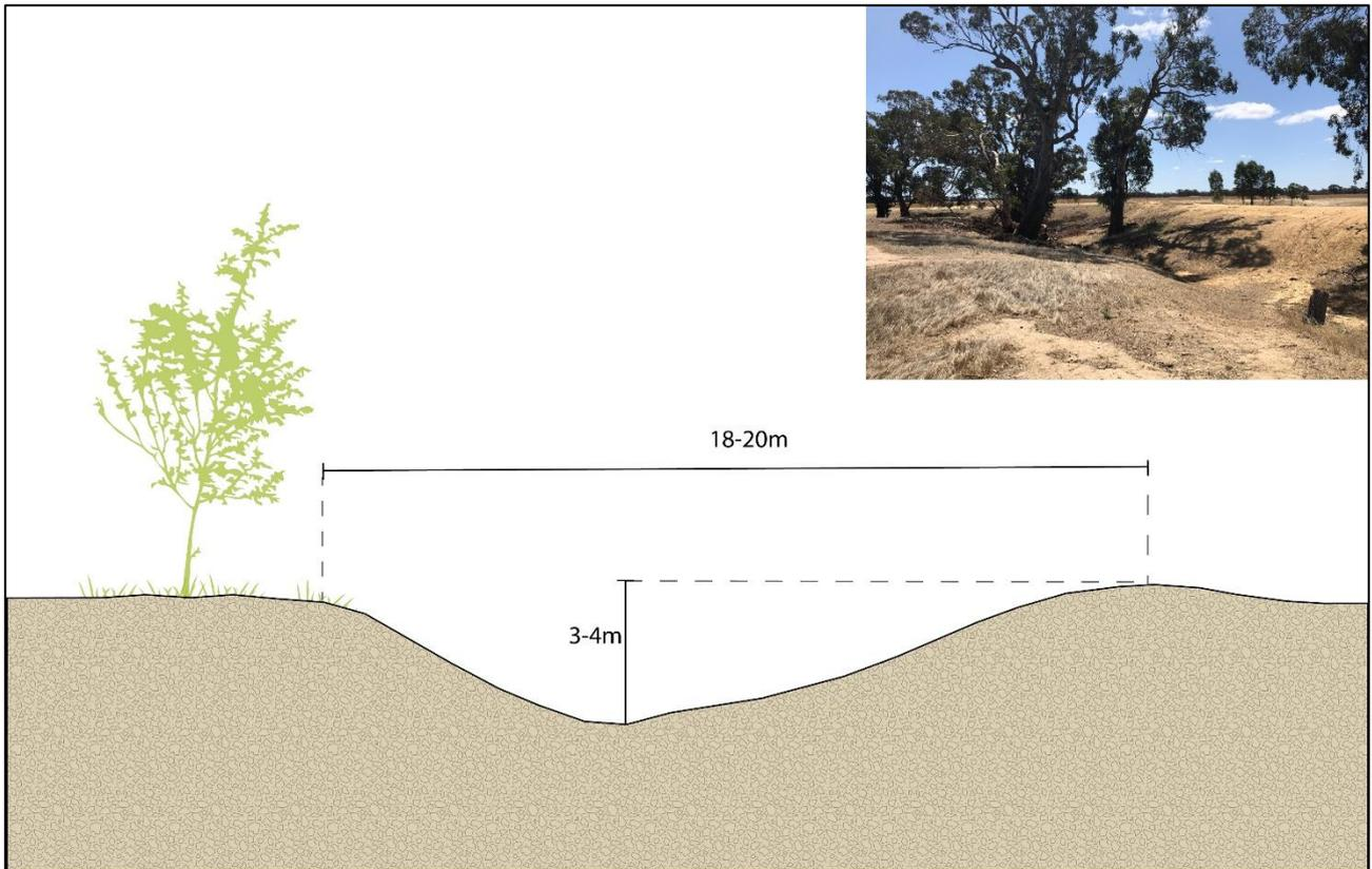
**FIGURE 5-5 TYPICAL CHANNEL DIMENSIONS IN THE UPPER REACH EXCLUDING WHERE THE CHANNEL INHERITS PALAEOCHANNELS OF THE WIMMERA RIVER.**
