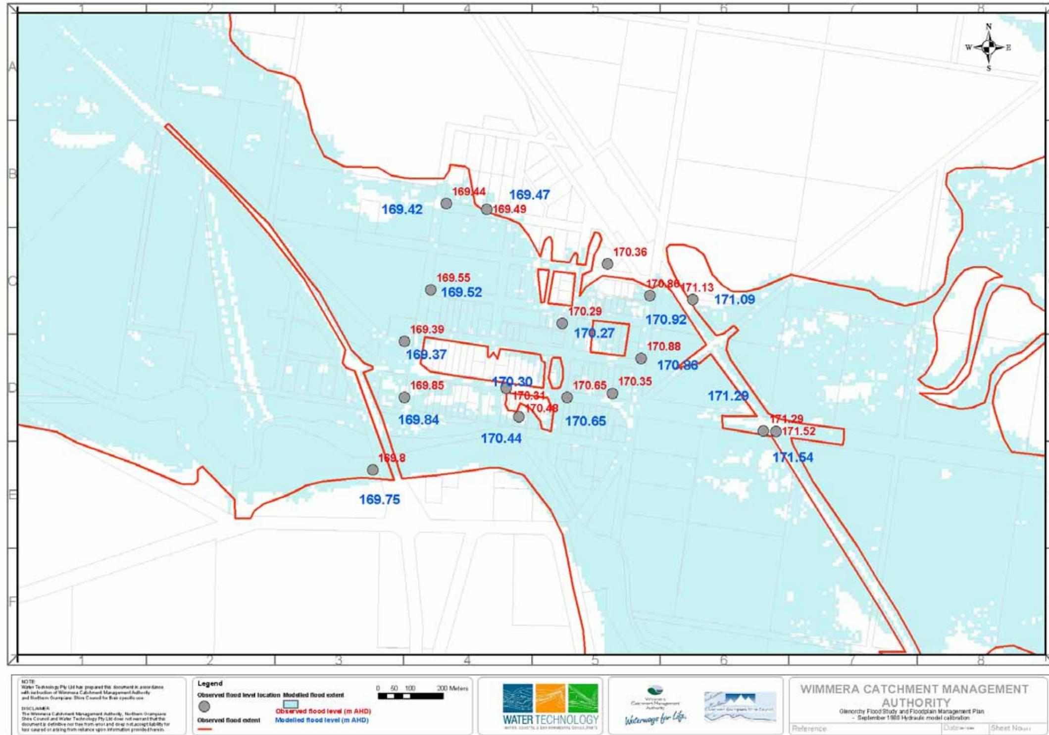
Figure 5-2 September 1988 flood event hydraulic model calibration
