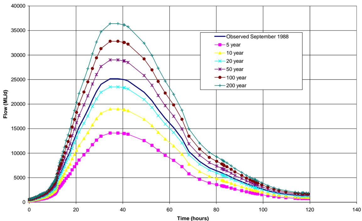
**Figure 4-3 Wimmera River at Glenorchy: Design flood hydrographs and September 1988 flood hydrograph**
