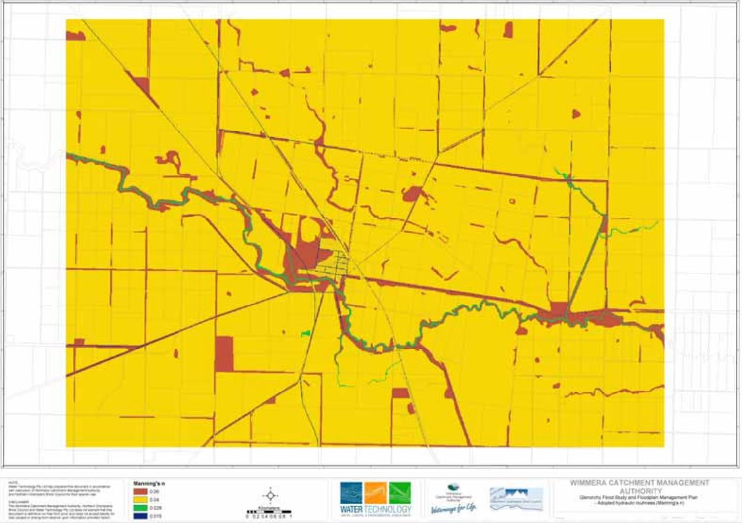
Figure 5-1 Initial Hydraulic Model Roughness
