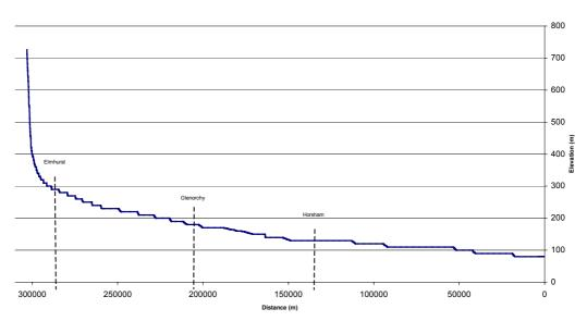
Figure D5 Wimmera River Longitudinal Profile
