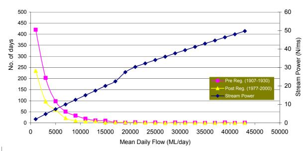
Figure A3.9 Flow Duration versus Stream Power – Downstream Horsham
