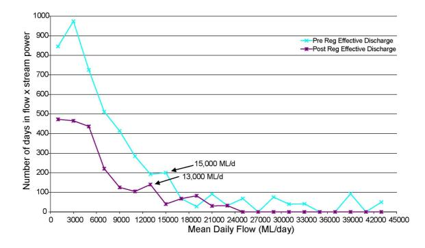
Figure A3.10 Effective Discharge Analysis – Downstream Horsham
