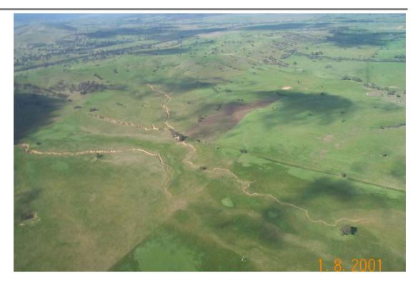
Severe gully erosion floods out at reduction of slope, depositing sediment
