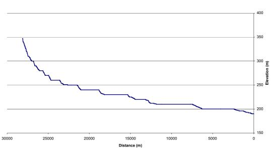
Figure D3 Seven Mile Longitudinal Profile
