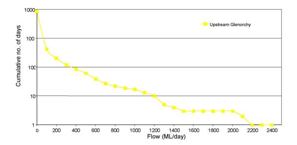
*Figure A3.4* Flow Duration Curve Wimmera River – Upstream of Glenorchy (415 206 and 415 237)
