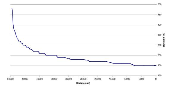
Figure D1 Wattle Creek Longitudinal Profile
