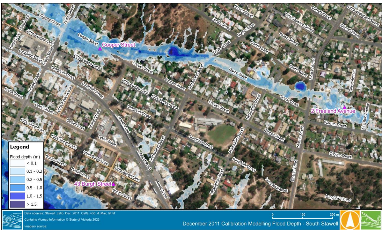
Figure 3-14 December 2011 calibration modelling flood depth – south Stawell
