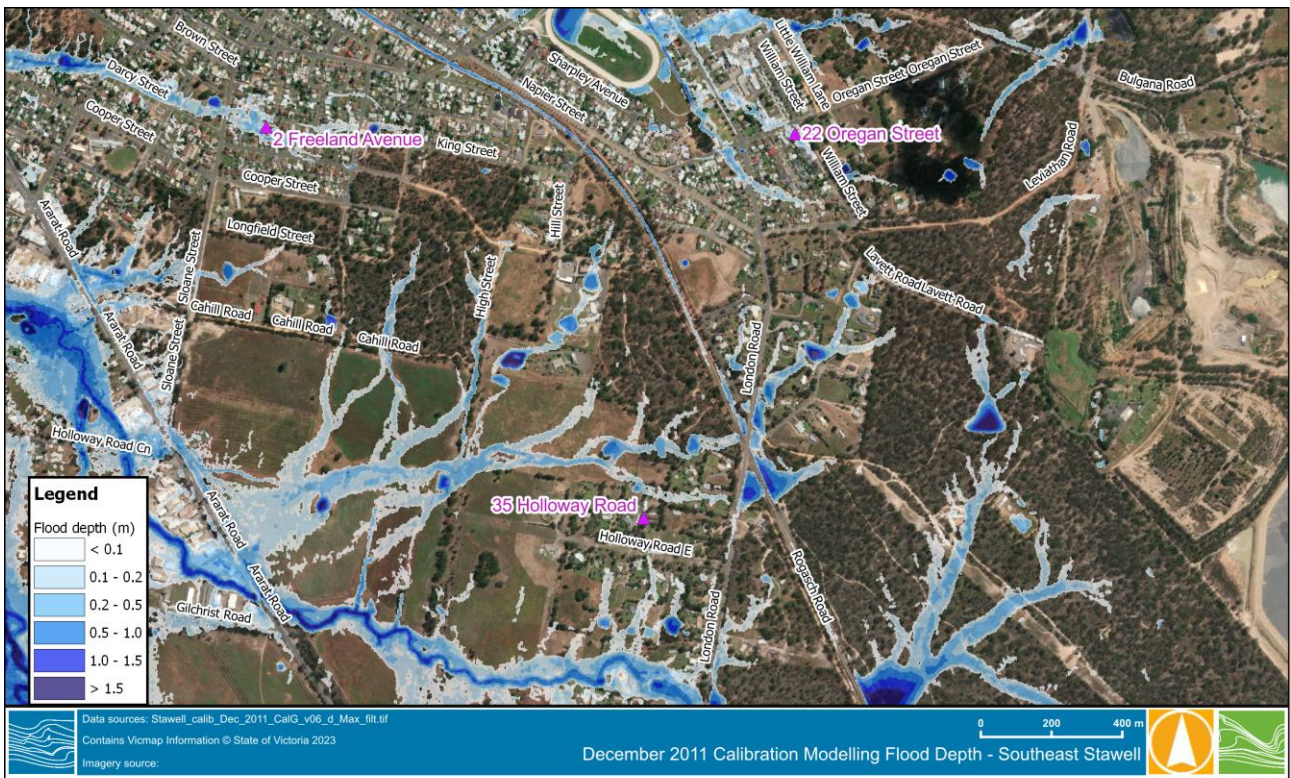
Figure 3-15 December 2011 calibration modelling flood depth – east Stawell
