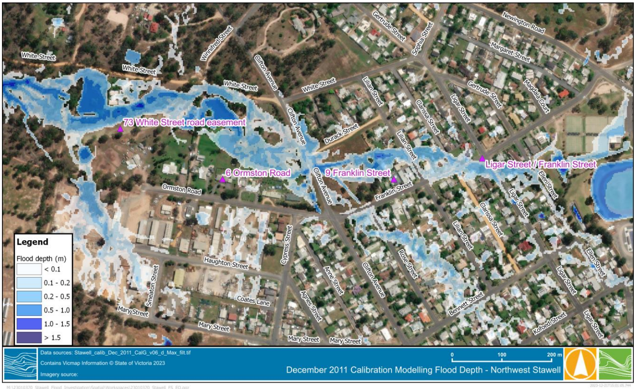
Figure 3-10 December 2011 calibration modelling flood depth – northwest Stawell
