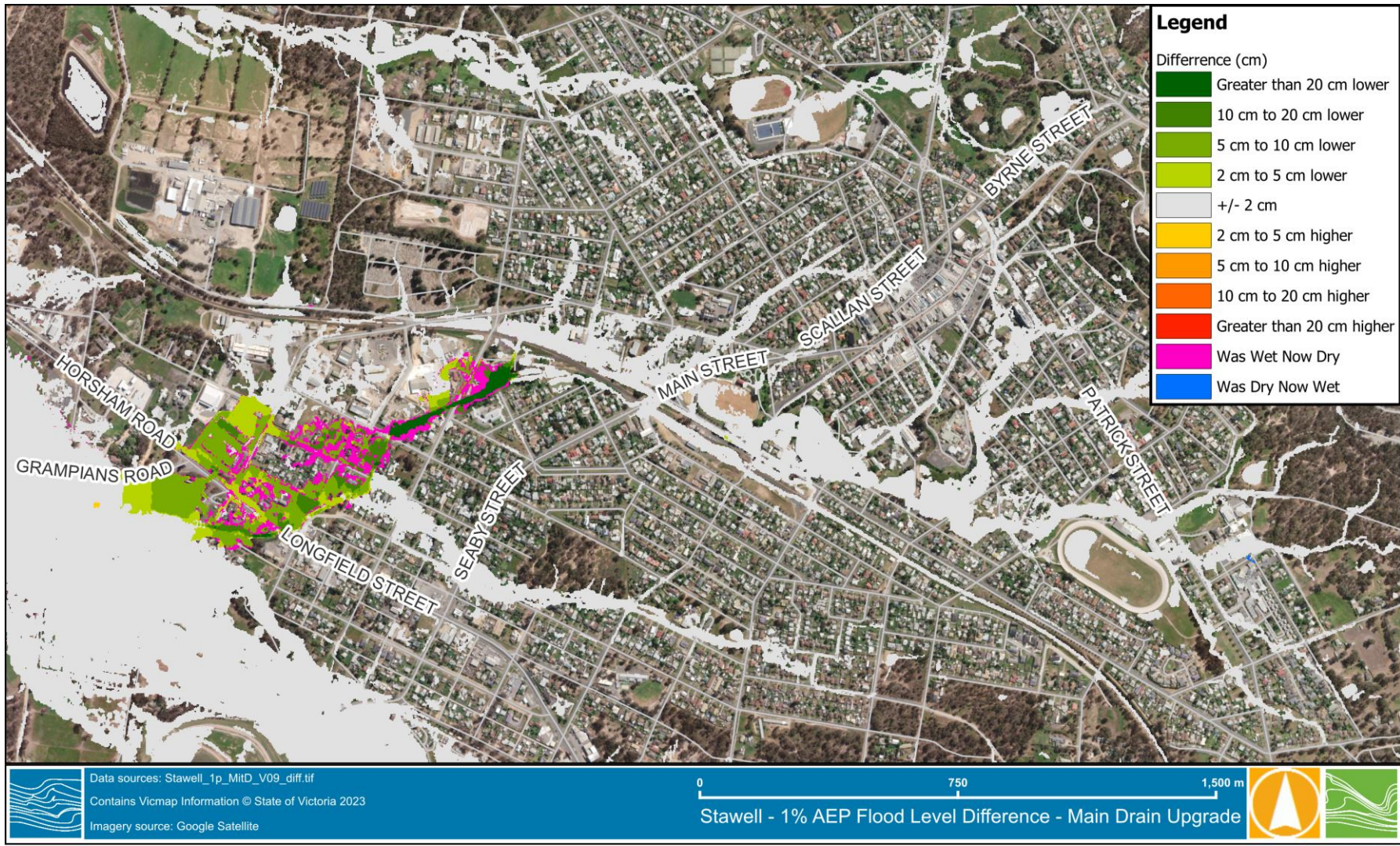
Figure 6-13 1% AEP flood level difference – Main Drain upgrade
