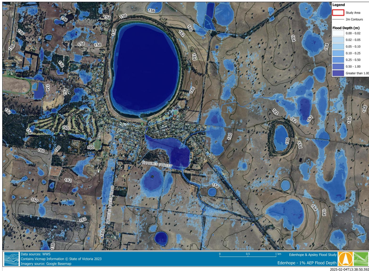
Figure 4-5 Broad extent - 1% AEP flood depth with water surface elevation contours
