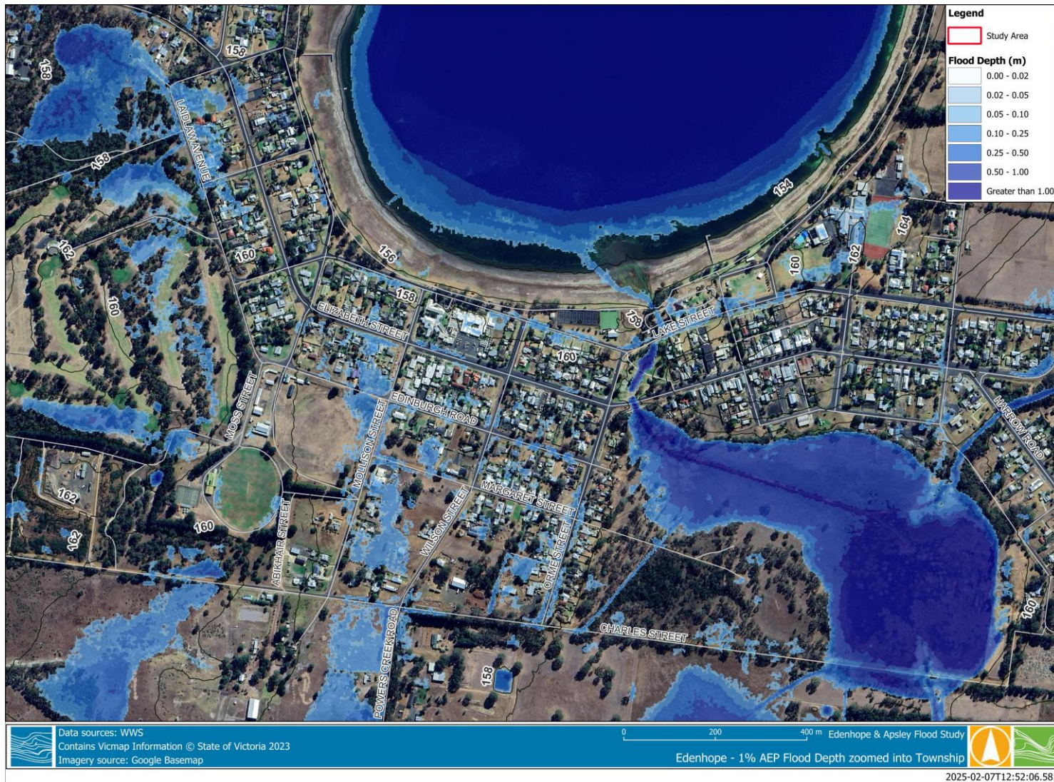
Figure 4-4 Zoomed into Edenhope - 1% AEP flood depth with water surface elevation contours
