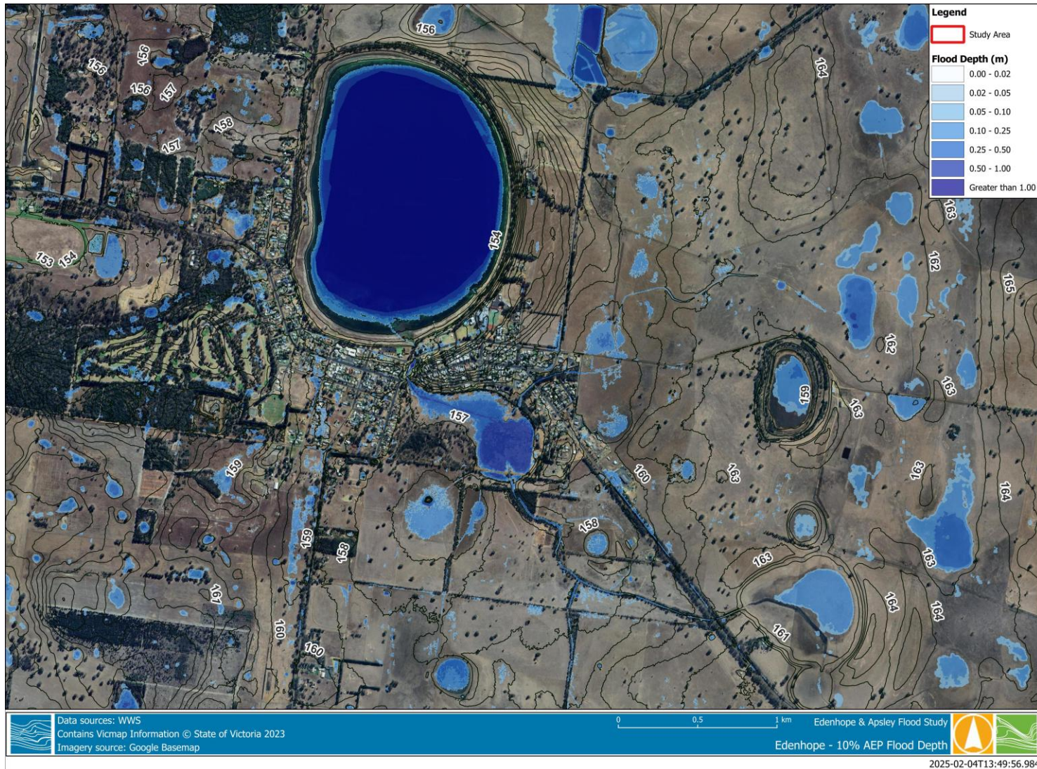
Figure 4-9 Broad extent - 10% AEP flood depth with water surface elevation contours
