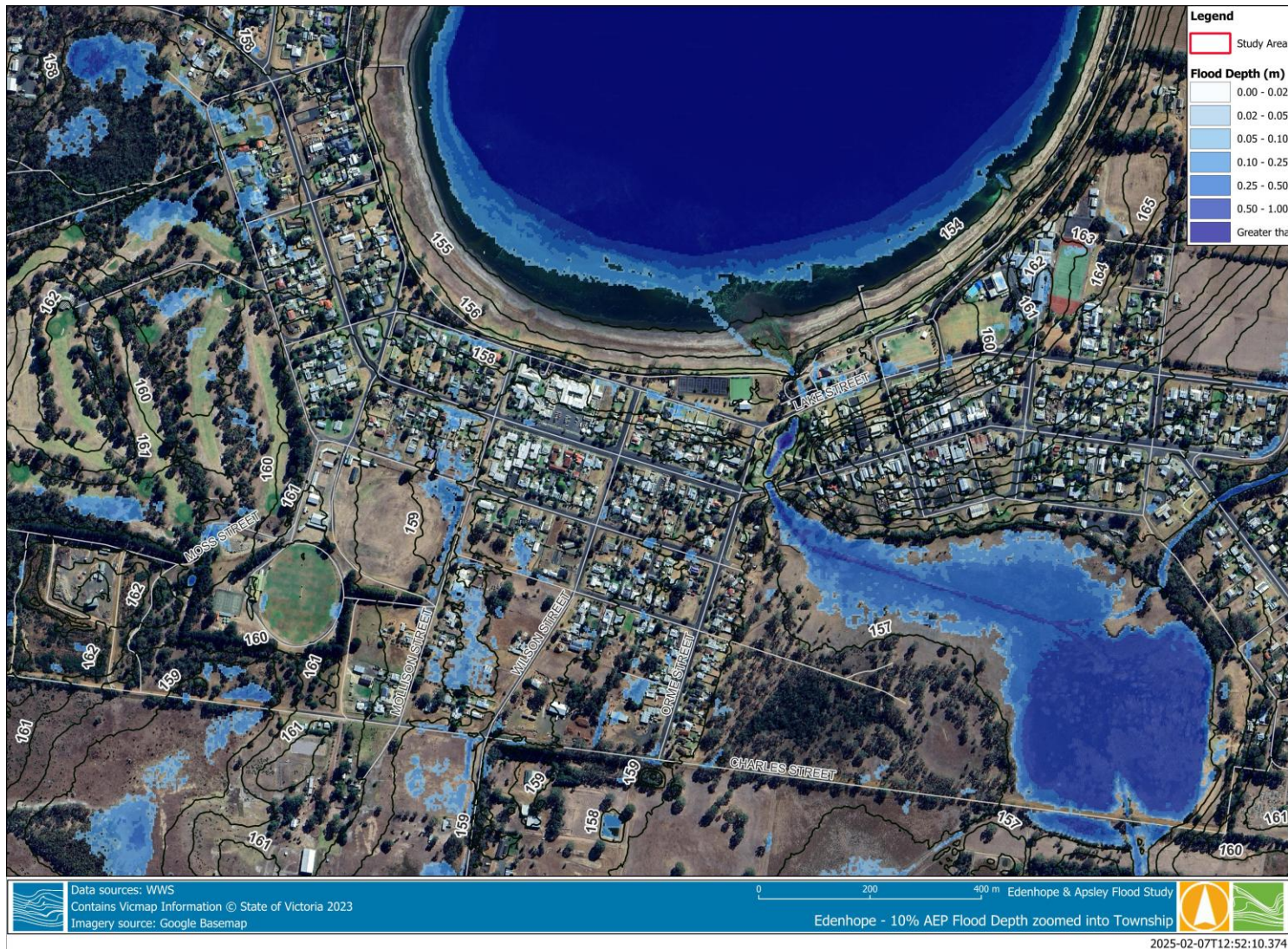
Figure 4-8 Zoomed into Edenhope - 10% AEP flood depth with 1m water surface elevation contours
