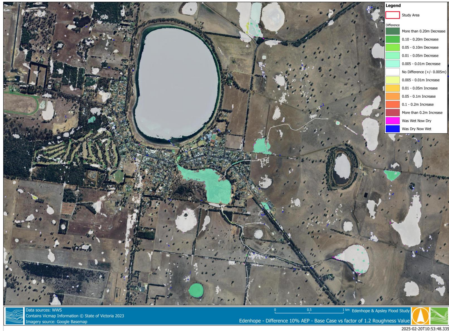
Figure 3-12 Difference Plot for 10% AEP – Base Case vs factor of 1.2 Roughness Value
