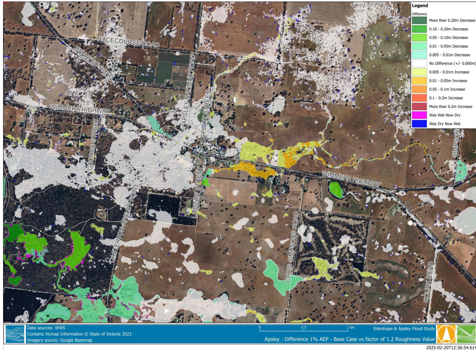
Figure 3-13 Difference Plot for 1% AEP - Base Case vs factor of 1.2 Roughness Value
