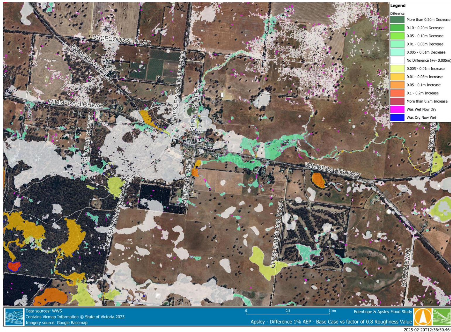
Figure 3-11 Difference Plot for 1% AEP - Base Case vs factor of 0.8 Roughness Value
