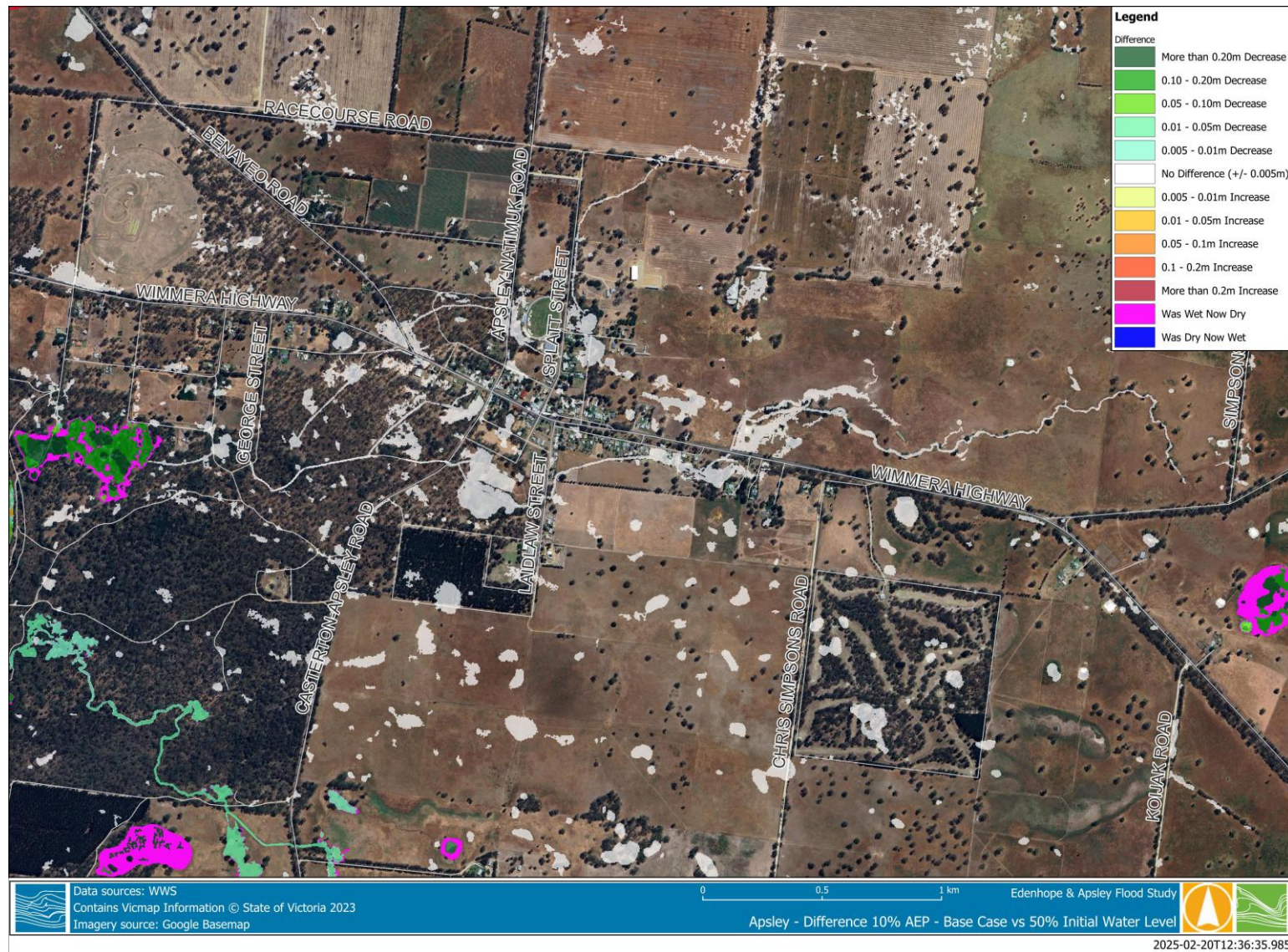
Figure 3-4 Difference Plot for 10% AEP - Base Case vs 50% Initial Water Level
