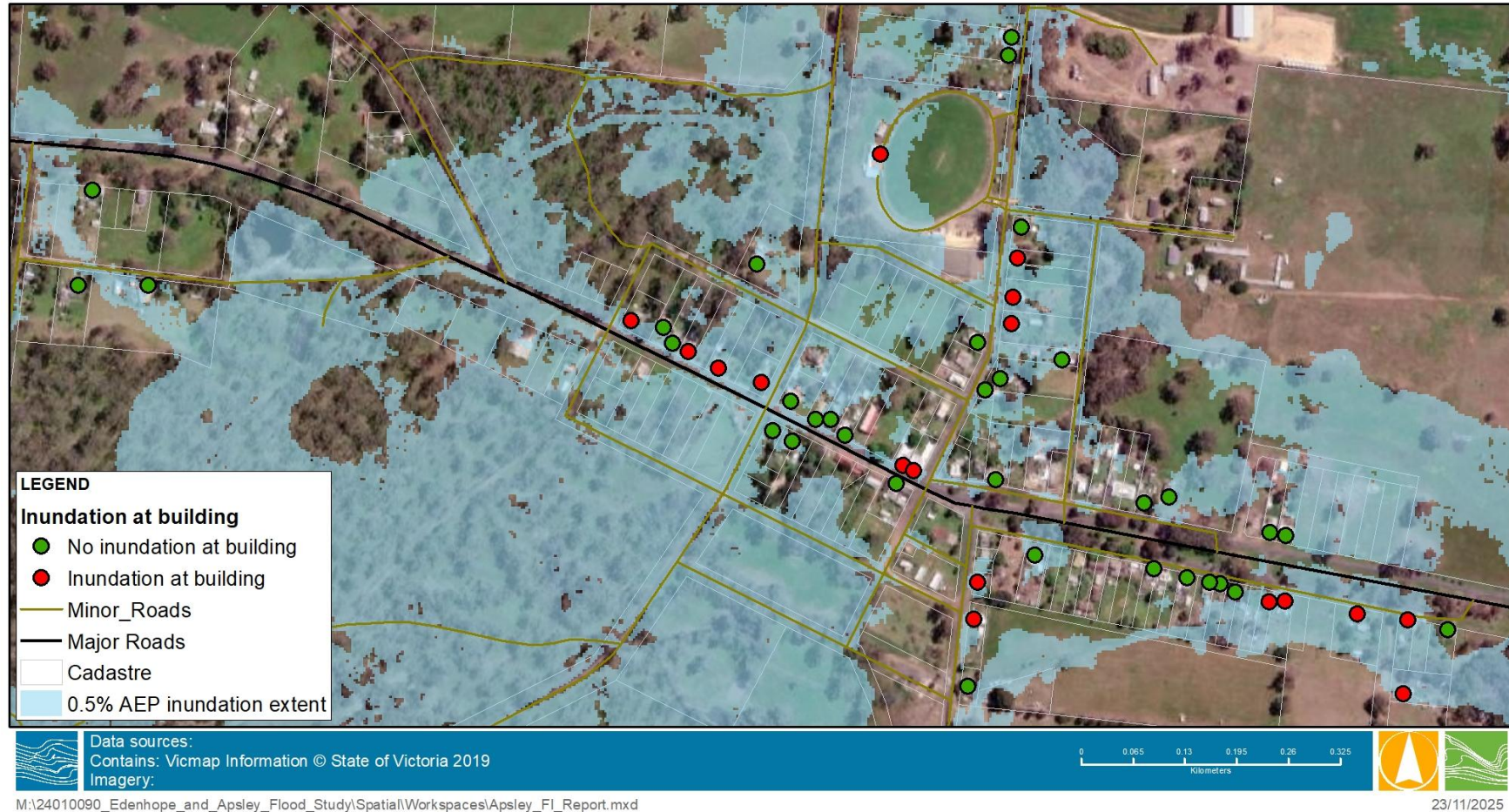
Figure 4-9 0.5% AEP - buildings inundated below floor
