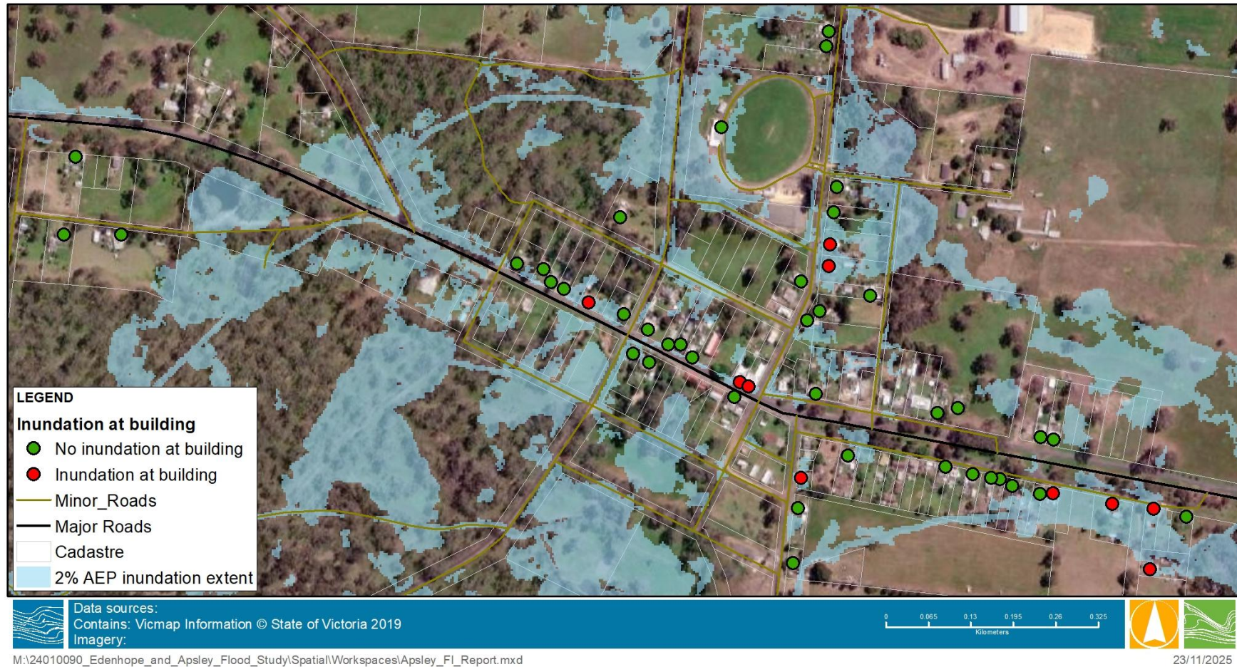
Figure 4-7 2% AEP - buildings inundated below floor
