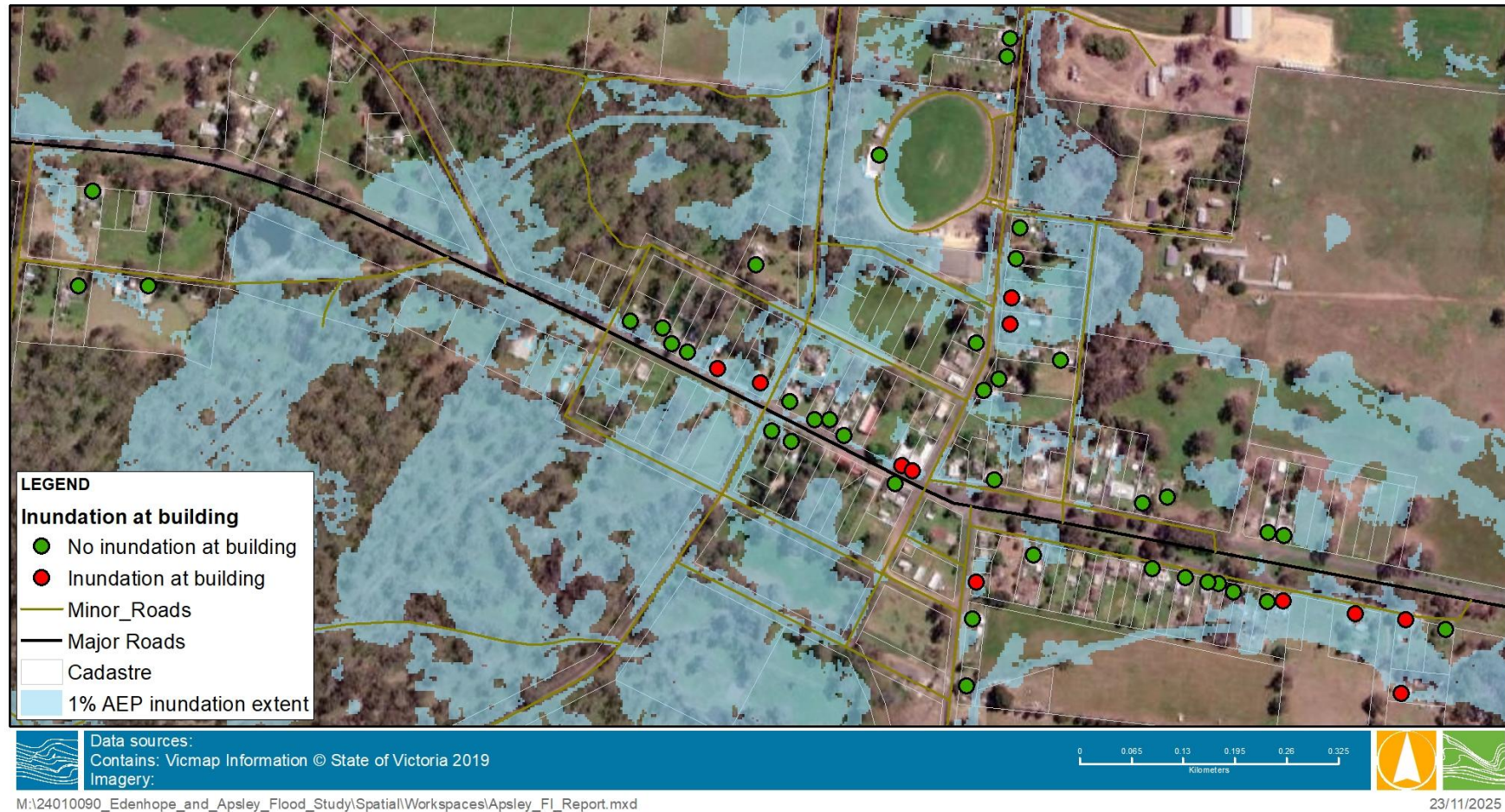
Figure 4-8 1% AEP - buildings inundated below floor
