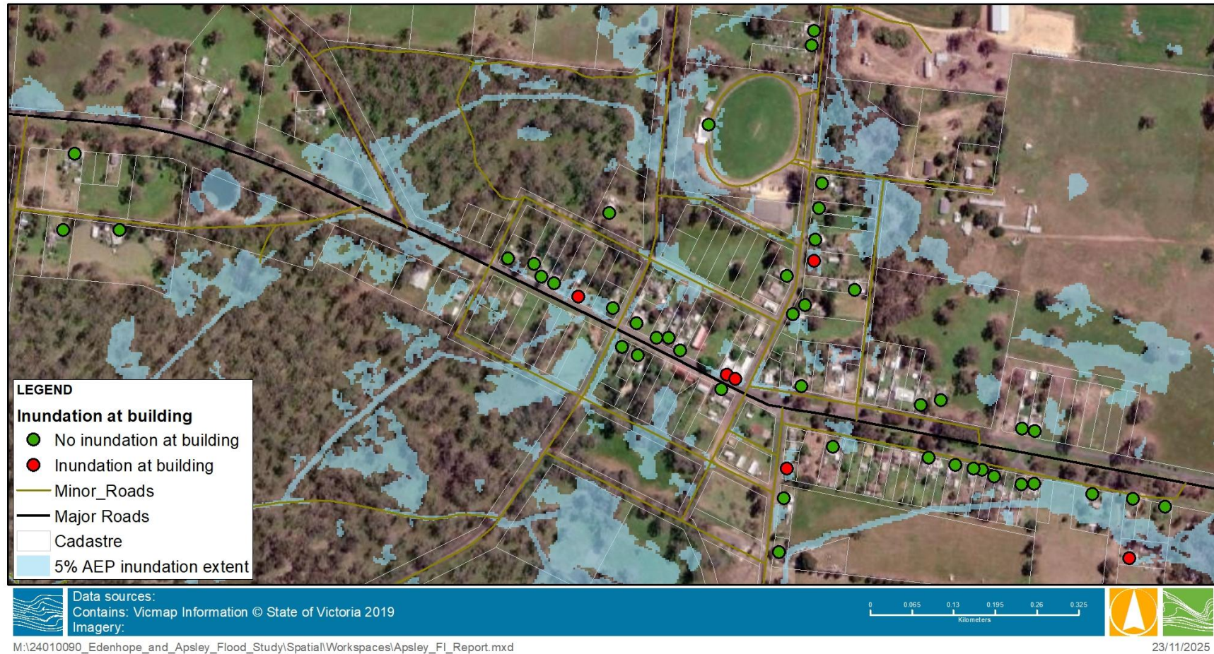
Figure 4-6 5% AEP - buildings inundated below floor
