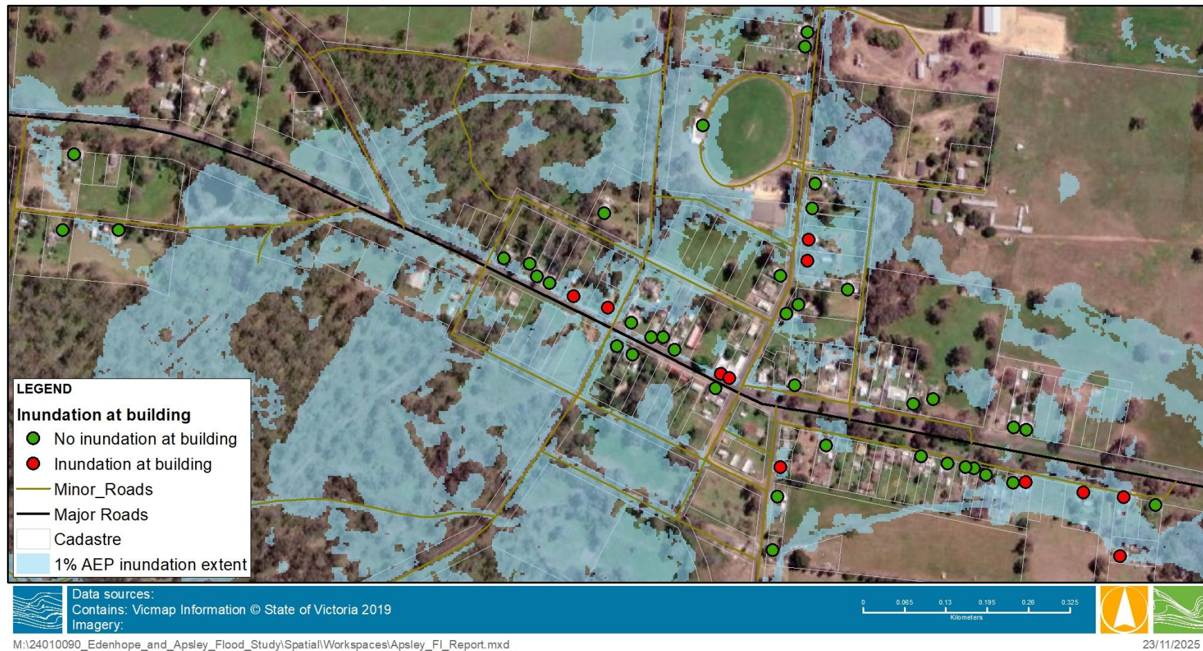
Figure 4-4 1% AEP - Buildings inundated below floor level
